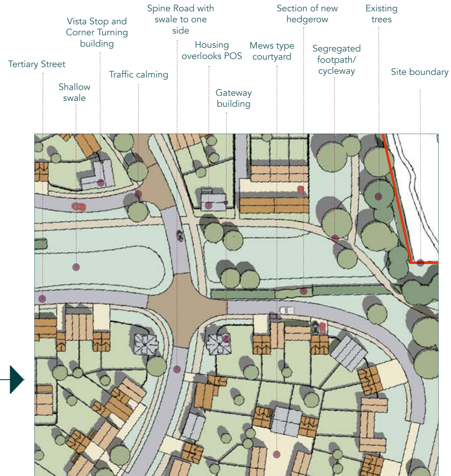
Fig.35 Detailed Plan of Mill Side Eastern Edge Sample Area - indicating scale, form and character
