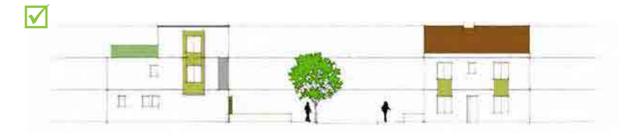
Proportions of elevations and their details should align. Colours, materials and textures should be harmonious. Street treatment should be similar in scale and articulation.
